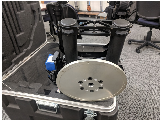
Figure 4.2: Custom mounting plate bolted on to the MōVI XL.
